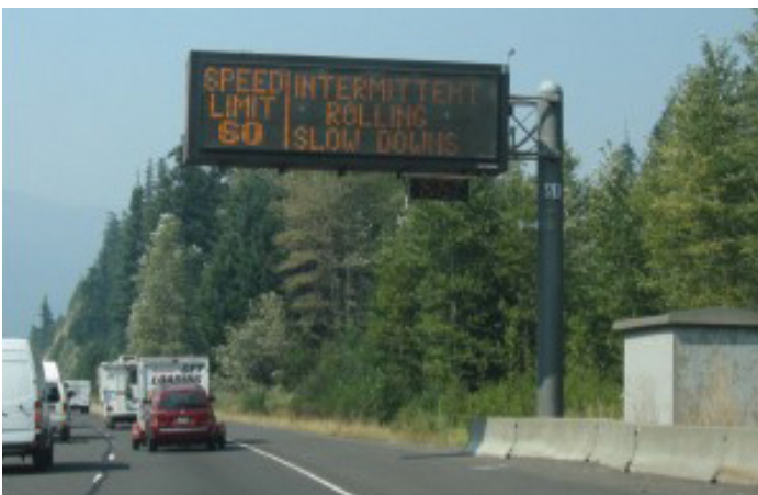
Existing permanent CMS in the area of a rolling roadblock operation can be used to supplement temporary public outreach tools during rolling roadblock operations. (Source: WSDOT)
