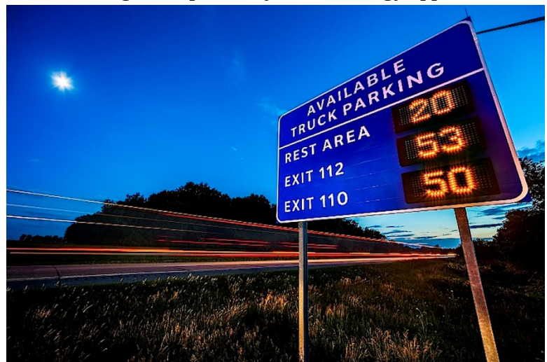
Figure 8. Photo. Truck parking information and management system on I-94 in Michigan.
