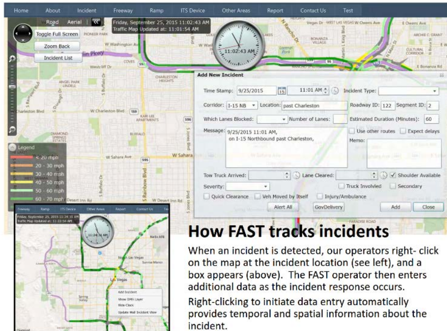
Figure 13: Screenshot. Snapshot of central software used by the Regional Transportation Commission (RTC) of Southern Nevada. (Source: RTC of Southern Nevada)
